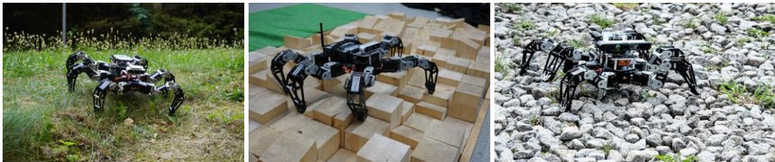
**Figure 3. UGV-Hexapod robot:** Operating in different terrains.
