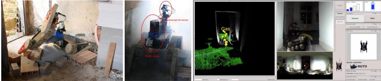
**Figure 1. UGV-VRAS robot:** tracked-robots equipped by flippers (left), its sensor suite (middle) and human interface (right).
