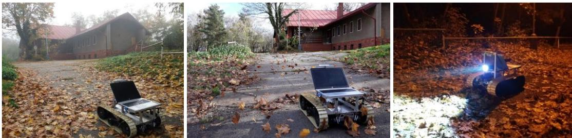
**Figure 2. UGV-Cameleon robot:** Operating in adverse conditions (fog, gale, night).
