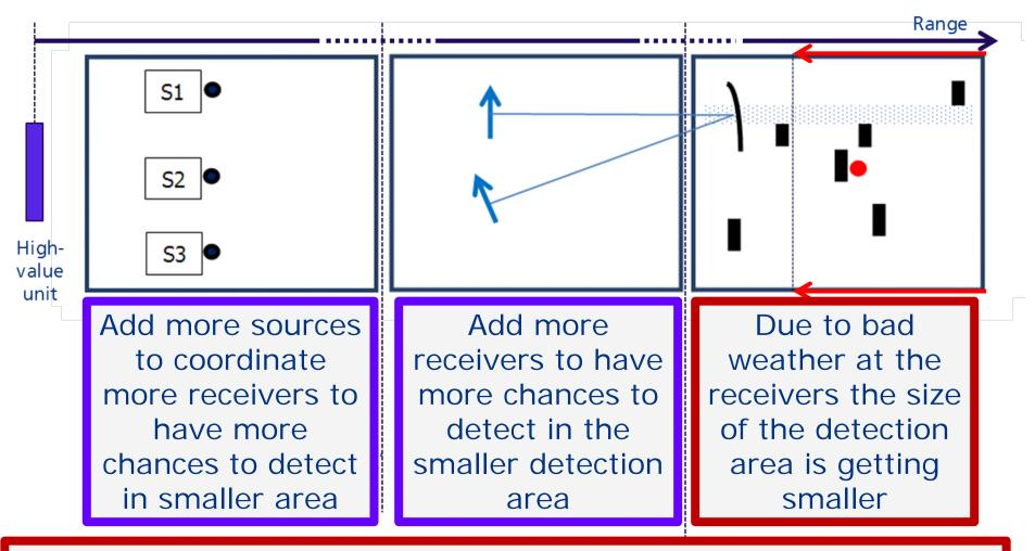
→ Calculation of how many sources and receivers are needed via adding independent surveillance layers to compensate for smaller detection area
