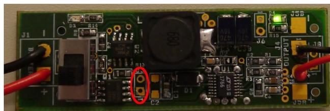
Figure 3: Additional pins for the power source of the regulator without undervoltage switch.
