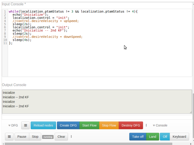
Fig. 3. Urbscript console. On the top – script editor, middle – output of executed script, bottom left – script execution control (surrounded with other controls of X-Copter Studio).
